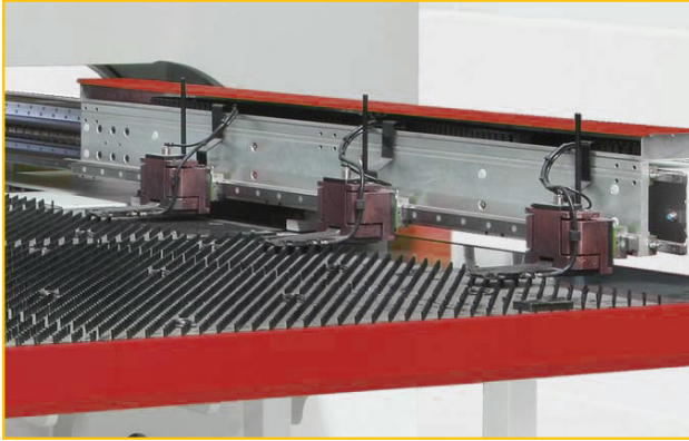
3 automatic repositioning sheet metal holding clamps.
