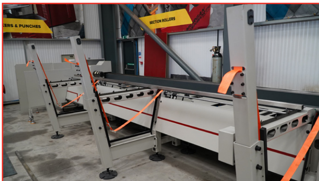
DUAL LOADING SYSTEMS
