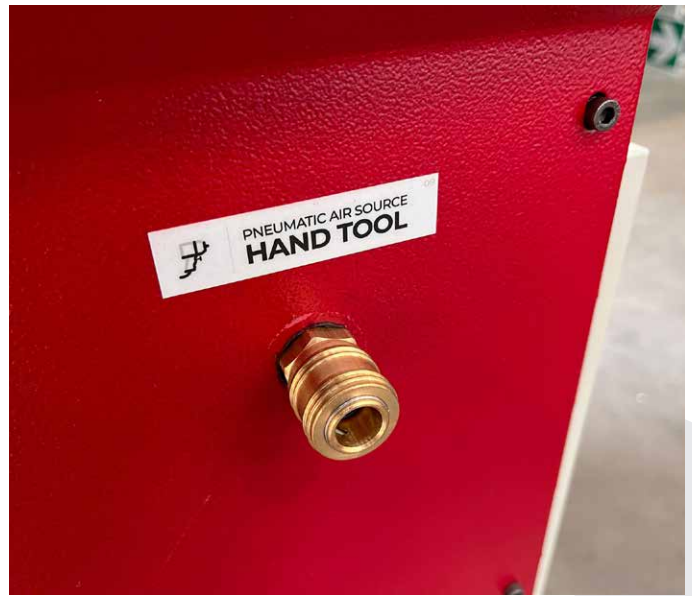
Compressed air outlet for operator tools
