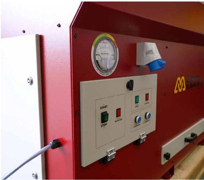
Controller with filter pressure gauge and 240V tool outlet
