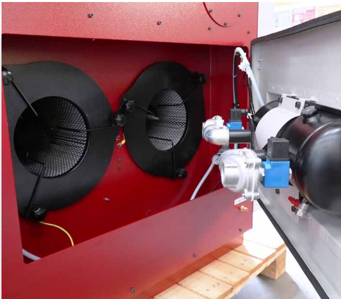
Filters and compressed air tank
