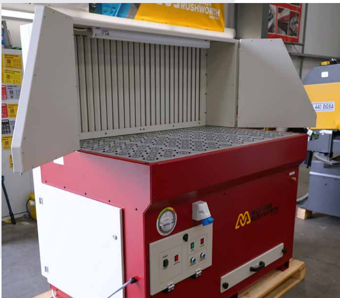
Lift catch and open wings for larger work pieces
