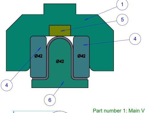
Part number 1: Main V Die for All Clamps Part number 5: Gas Spring Holder Part number 4: Special Punch for s4 Ø42 H50 Clamp Part number 6: Ø42 Punch
