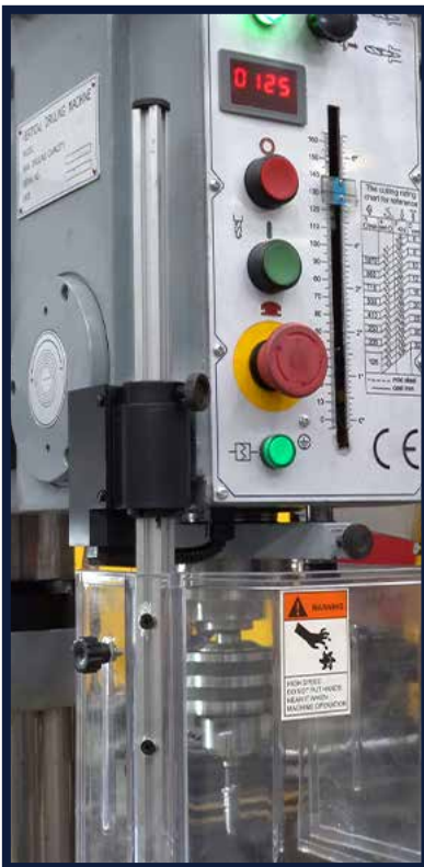
RPM DIGITAL READ-OUT (AVAILABLE ON SR32AE, SR50VAE, SR50TAE & SR70TAE)
