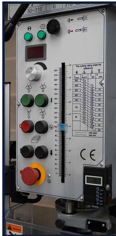
SR50VAE CONTROL PANEL WITH VARIABLE DRILLING DEPTHS
