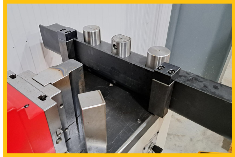
Flat bar straightening tool.
