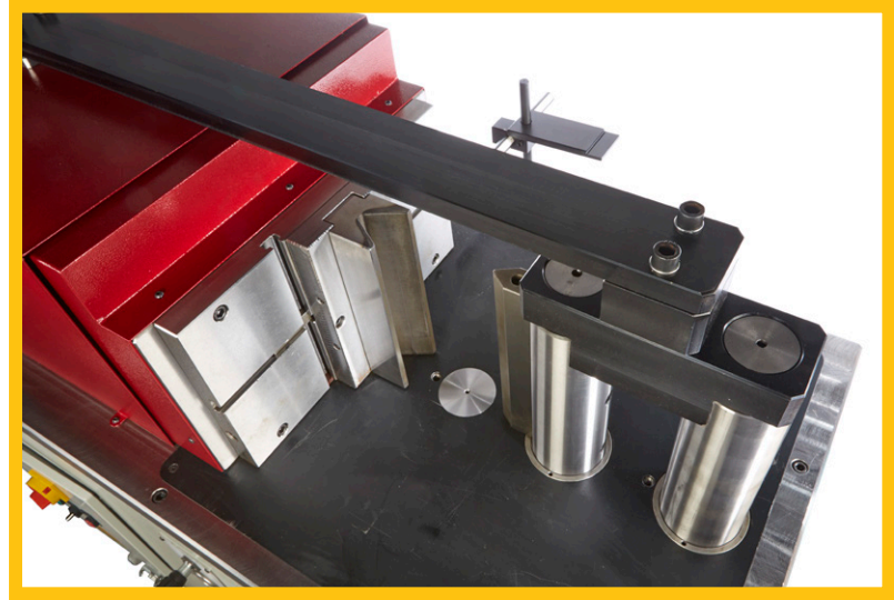
Standard tooling with anti-deflection bar.
