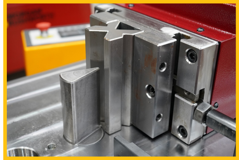
A 30° bolt punch, paired with a multi-way v-die for tighter than 90° folds.
