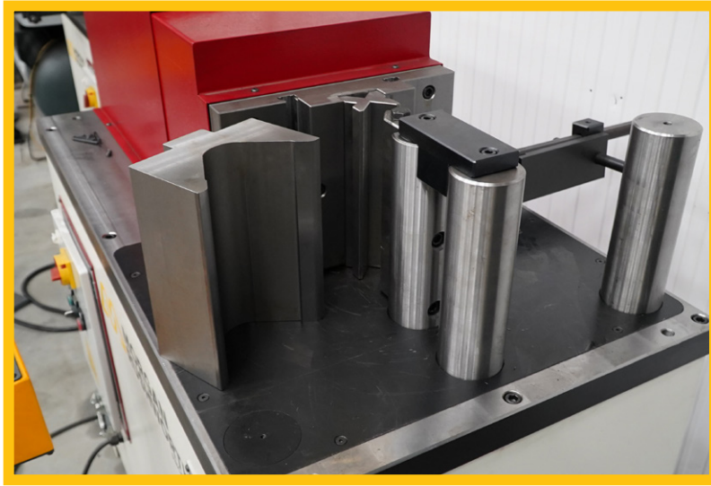
Larger V dies for bending thicker plates
