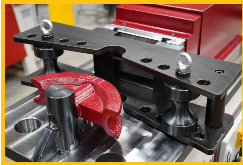
2 jaw bending tool for thick wall pipes up to 90°.
