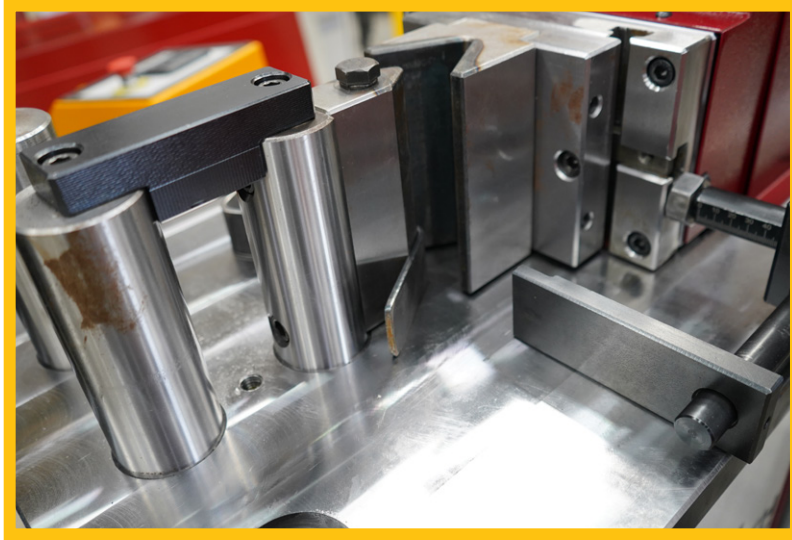
The standard tooling for all HBMs is a v-die and punching tool.
