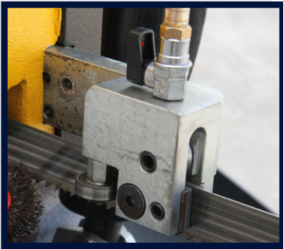
FLOOD COOLANT SYSTEM
