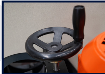
MANUAL PIPE CLAMPING
