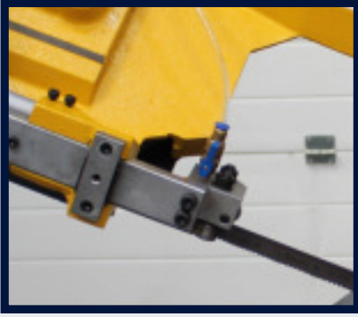
FLOOD COOLANT SYSTEM
