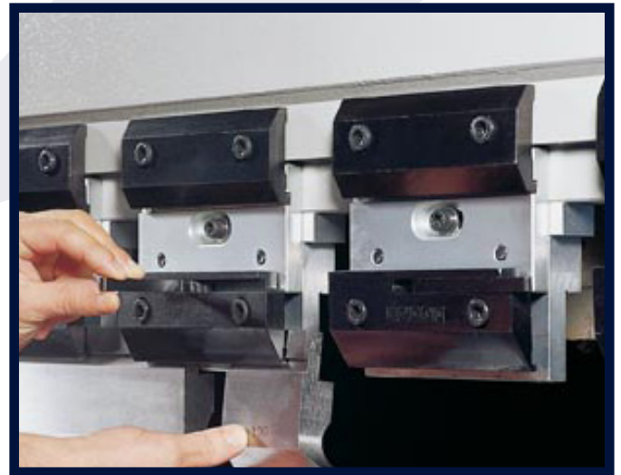
QUICK RELEASE TOP TOOLING (OPTIONAL)
