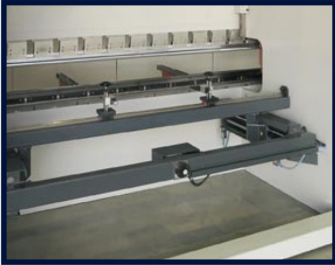
X AXIS CNC BACKGAUGE
