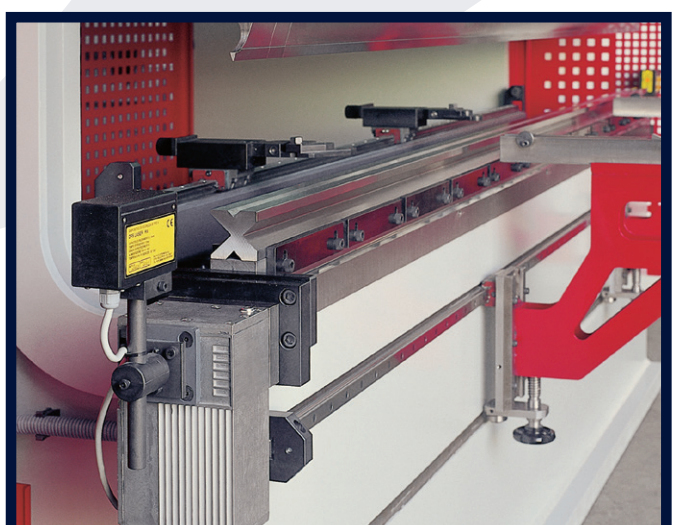
CNC CONTROLLED BOTTOM TOOL CROWNING SYSTEM (OPTIONAL)
