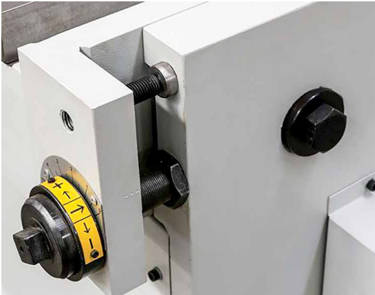
BLADE GAP ADJUSTMENT
