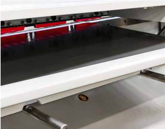
STANDARD BACK GAUGE SYSTEM
