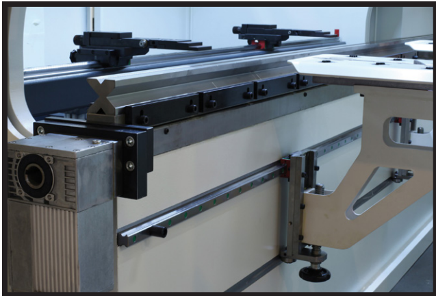
CNC Controlled Bottom Tool Crowning
