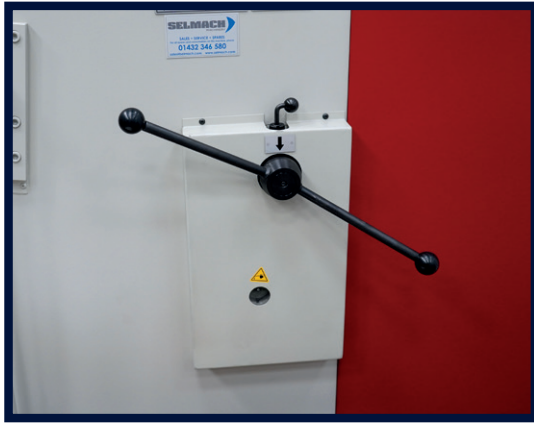
MANUAL BLADE GAP ADJUSTMENT
