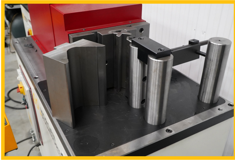
Larger V dies for bending thicker plates
