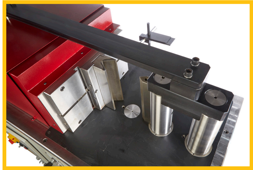
Standard tooling with anti-deflection bar.
