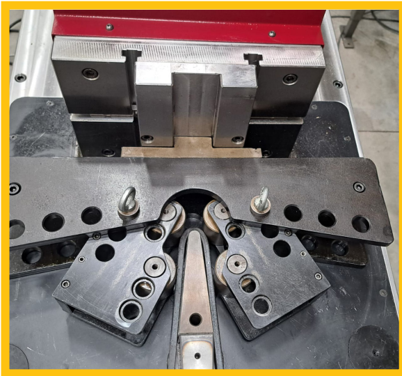
4 jaw bending tool with 30° bolt punch for bending specific profiles.
