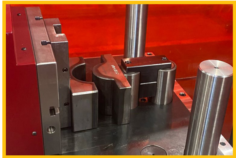
Pipe clamp pressing and forming tool for flat bar bending.
