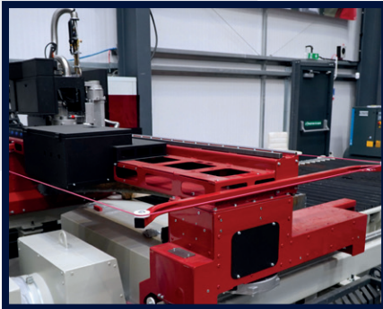
WIDE GANTRY PROVIDES CUTTING STABILITY
