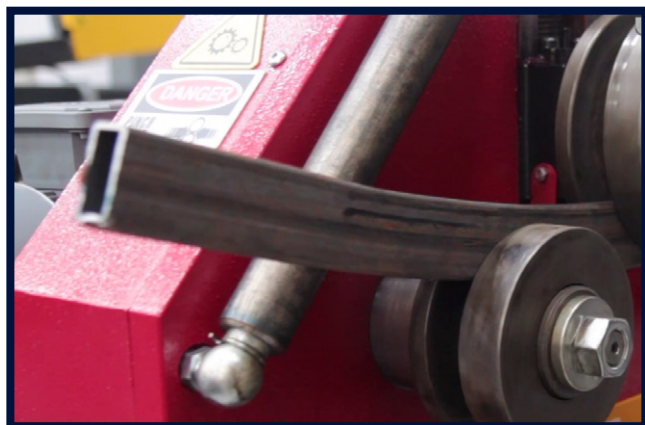
BENDING BOX SECTION
