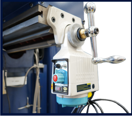
POWER FEED UNIT
